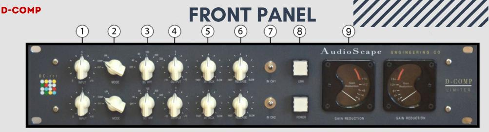
(1) Input - Input level, passive (trimming) from 1-5 and then active (boosting) from 6-10. There is some harmonic distortion available here in which the clipping can be a useful tool for transient control.
